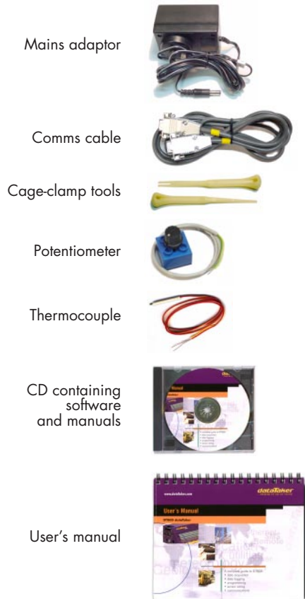
FIGURE 7 Accessories supplied with your DT800 (plus the user's guide you're reading now)
